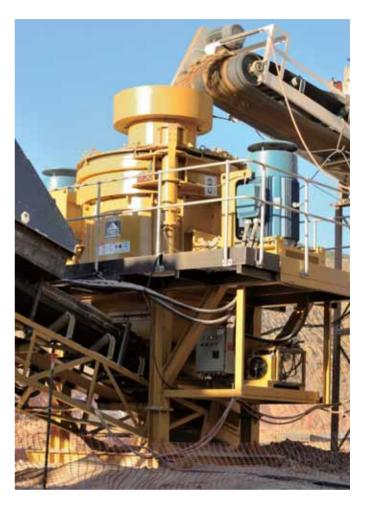
Modular Vertical ShaftImpact Crusher Stations include feedboxes and discharge chutes that incorporate dust control plenums. Convenient accessible work platforms and stairways provide operator safetyand ensure simple service and maintenance.
