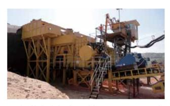
Optional hydraulic breaker modular support structures can be pair with these primary stations to effectively manage oversized feed. Operator control rooms or towers can also be supplied as stand-alone control modules or as extensions to overall plant motor control centers.
