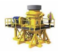
TRIO's TC-Series Cone Crushers unitize a time proven design platform that has been optimized with robust mechanical components and labor saving user friendly operating features. The TC-Series Conesare a combination of quality, performance and reliability for secondary and tertiary crushing applications.
