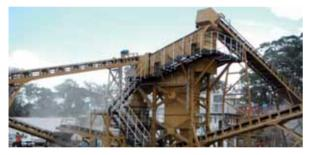
Safe and accessible work platforms are built with grated walkways, stairways, hand rails, knee rails and toe plates that can be tailored to satisfy local dimensional requirements. Operator friendly stairs are provided to ensure user maintenance and service access.
