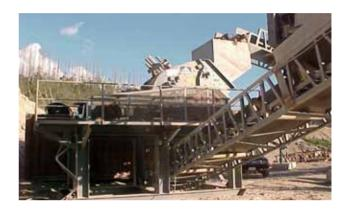
Hydraulic breaker modular support structures are available in these primary stations to effectively manager oversize feed. Operator control rooms and towers can also be supplied as stand- alone control modules or as extensions or overall plant motor control centers.
