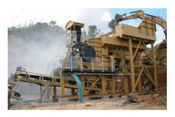
TRIO designs include both sloped side and rock box style hoppers in a variety of configurations. Safe and accessible work platforms are built with grated walkways, stairways, handrails, knee rails and toe plates. These features can be tailored to satisfy local dimensional requirements.
