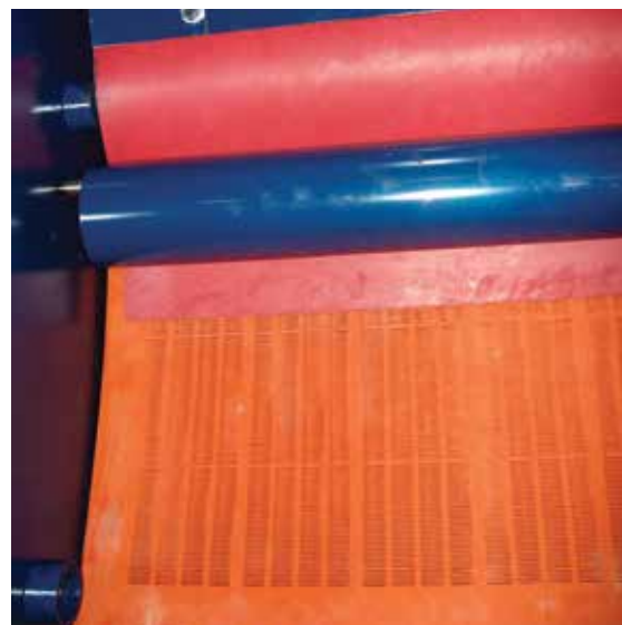
Enduron® sieve bend with manual adjust and Linatex® polyurethane screen media
