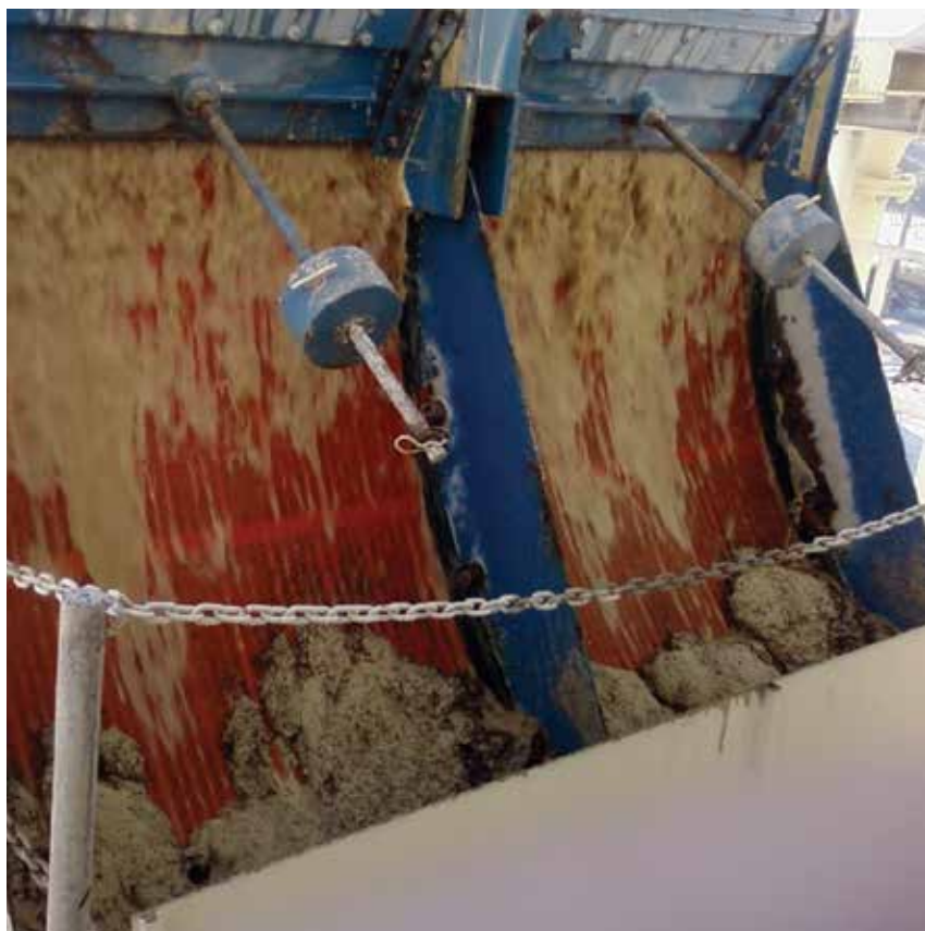
Sieve bend with a counter weight, feed spreader and Linatex® polyurethane screen media
