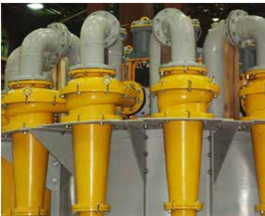
Each cluster of Cavex® hydrocyclones is modelled using the latest 3D CAD technology
