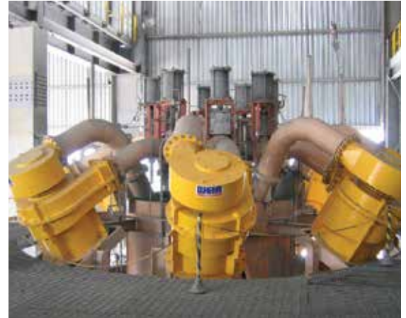
Cavex® hydrocyclones fitted with Air Core Boosters in operation in a facility in Brazil.
