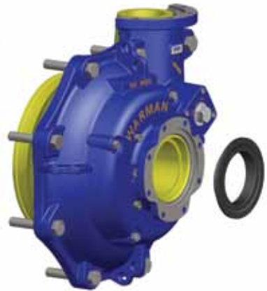
Quick and easy disassembly: Front sub-assembly easily removed for maintenance - volute liner attached to cover plate. Four camlocks hold liner into cover plate. No troublesome threads.
