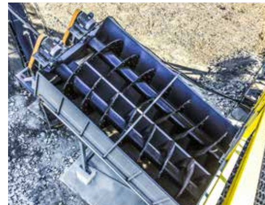
TWIN DEWATERING SCREWS
