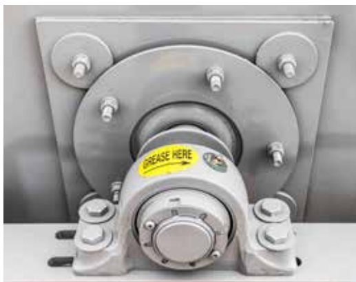
SLINGER PROTECTS LOWER BEARING
