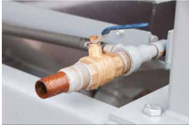
SPRAY NOZZLE FOR DISCHARGE CLEANOUT
