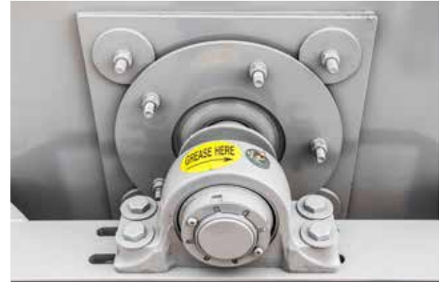
SLINGER PROTECTS LOWER BEARING
