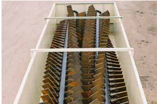
SPIRAL PADDLES FOR CONTINUOUS AGITATION
