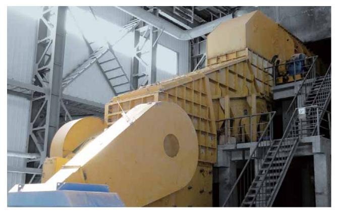
TRIO apron feeders are individually designed for your specific application. We take into account a host of variables; such as load surcharge height, material characteristics, maximum lump size, and loading method. This attention to detail in design and the highest quality components insures minimal down time and lowest overall operating costs.
