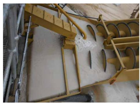
The sand particles are transported to the inclined discharge end by a double pitched steel spiral shaft equipped with replaceable cast wear shoes. The smaller lighter unwanted particles are floated to the surface of the claim settling pool and are discharged over the weirs.
