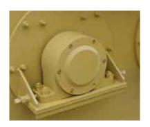
All TRIO Washers utilize a lower outboard grease lubricated, anti-friction, self-aligning spherical roller bearing assemblies with replaceable rubber "donut" seals and stainless steel wear sleeves. The mounting of the bearing outside the tub protects the bearing from external water and dirt commonly associated with plant operations and provides easy inspection and fast maintenance.
