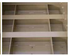
Deep ridged low carbon steel side frames and a thick feeder pan are fabricated and stress relieved with honey comb style reinforcement capable of absorbing and isolating tremendous shock loads.
