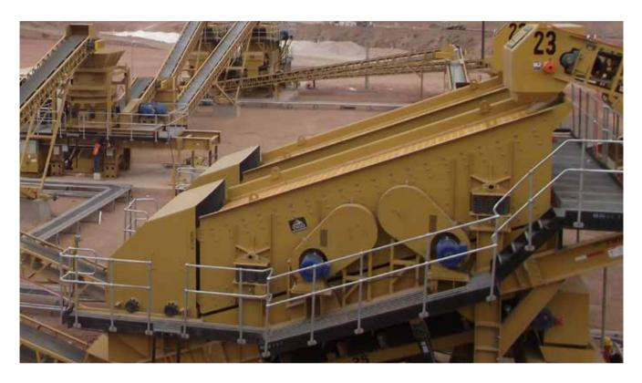
The TIO Series screens are designed for continuous operation in the most demanding applications and have a wide range of applications in both wet and dry operating scenarios with a feed acceptance size of 8". The operating inclination can be varied from 15 to 20 degrees depending on the velocity required to stratify the material.
