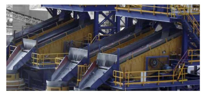
All components mounted to the screen side panels are attached with Huck bolts. The vibrating units are attached with threaded bolts for easy servicing. No welding is used; this process insures rigidity and structural integrity and eliminates stress fatigue in the screen body insuring a long productive service life.
