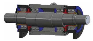
TRIO Pitman Shafts are forged high strength steel, fully CNC machined and precision ground at the bearing journals. The large frame and pitman self-aligning spherical roller bearings are closely spaced for maximum strength and extended service life.
