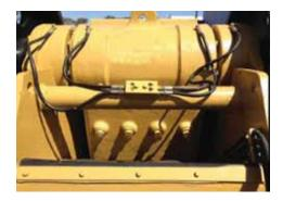
A conveniently located grease manifold allows easy access lubrication
