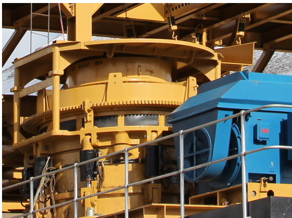
TRIO®TC6 new generation cone crusher operating at an Iron Ore mine in Northeast Asia.
