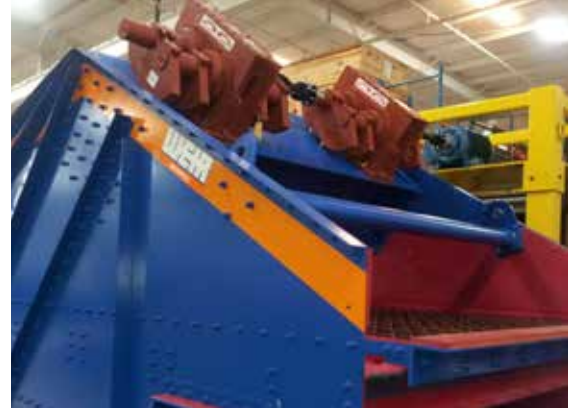
Screen motion provided by linear exciters
