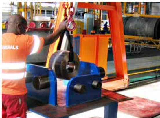
Weir Minerals exciter refurbishment
