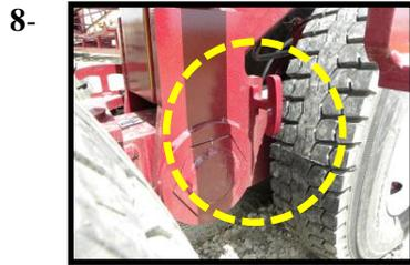
8- Lower Magnum back to the ground and Remove the retention pin (Left Picture) that prevents the walking beam from tilting and place it in the swing arm brace for storage (Right Picture).
