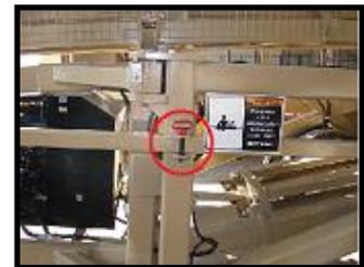
8- Manually swing the axle into radial position. Once in the radial position place the swing axle brace retention pin in the new position.
