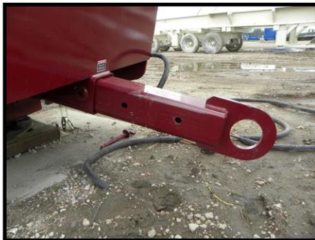
Extend the pintle hitch and attach a chain to the pintle hitch (Left) or to the circular lifting points (Right) in the frame of the convey tail.
