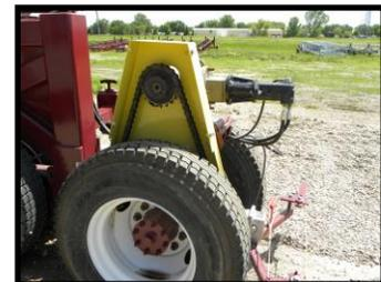
3- Bring the two ends of the chains together and insert the master link. Bring the master link in from the back and through the opening.
