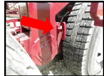
6- Lower the lifting jacks until both sets of wheel are slightly off the ground.
