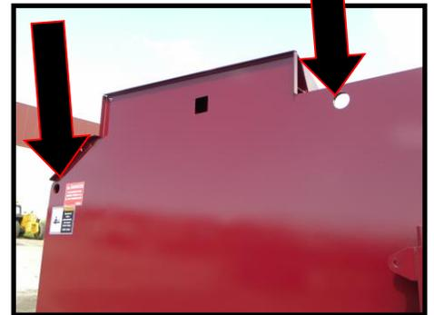
**It is important to use the designated lifting eyes for moving your conveyor. Failure to do so can result in equipment damage.**
