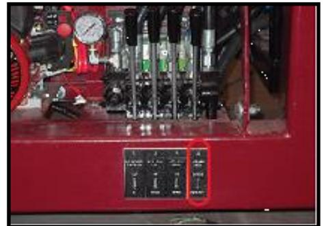
**PLEASE NOTE: Using the auxiliary gas powered hydraulic unit, the stinger can be extended partially to remove weight from tail while lifting off truck. Extending the Stinger will remove a substantial amount of weight from the tail making it easier and safer to unload.**
