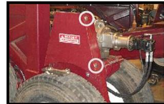
2- Remove the chain (s) from the black tool box mounted on the undercarriage. Wrap the chains around the lower sprocket and meet the two ends on the upper sprocket. Ends should meet near the opening in the back of the guard.
